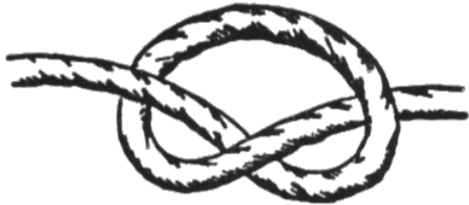
Overhand Knot - the basis of many knots
